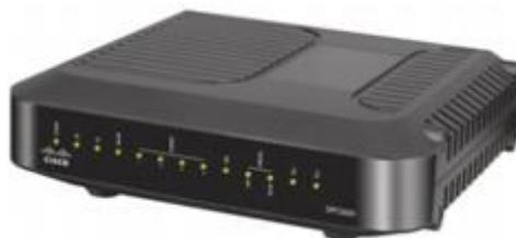
**Figure 4.** Modem Router
